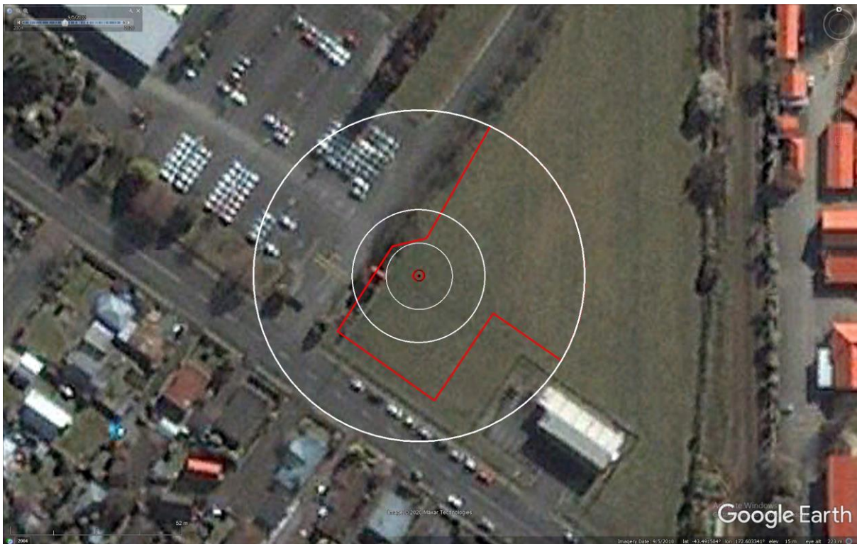
Figure 50: Absence of ejecta for Sep-10 EQ; evidence No. 2 – satellite image.
