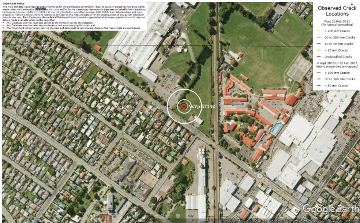
Figure 26: Absence of ground cracks indicating no lateral spreading for Canterbury Earthquake Sequence.
